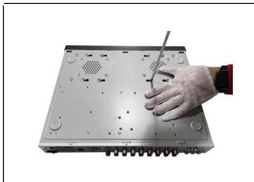
Figure 1-6 Fix the HDD
