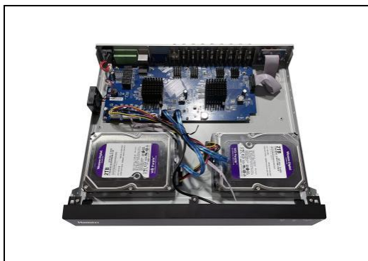
Figure 7 Connect the power and data cables
