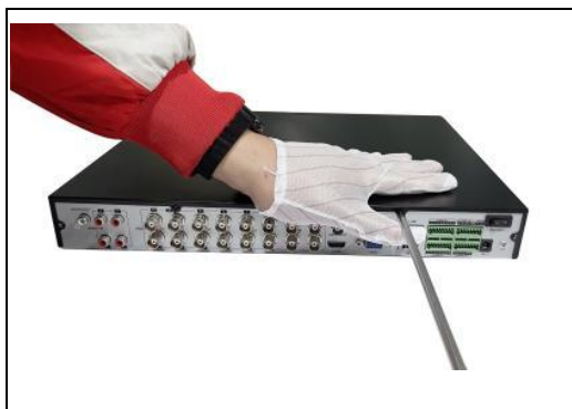
Figure 1-8 Install the cover and screws
